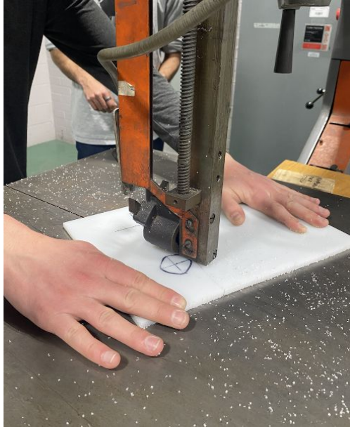
Used the vertical band saw to cut out shape of base Base made out of Teflon (food-safe)
