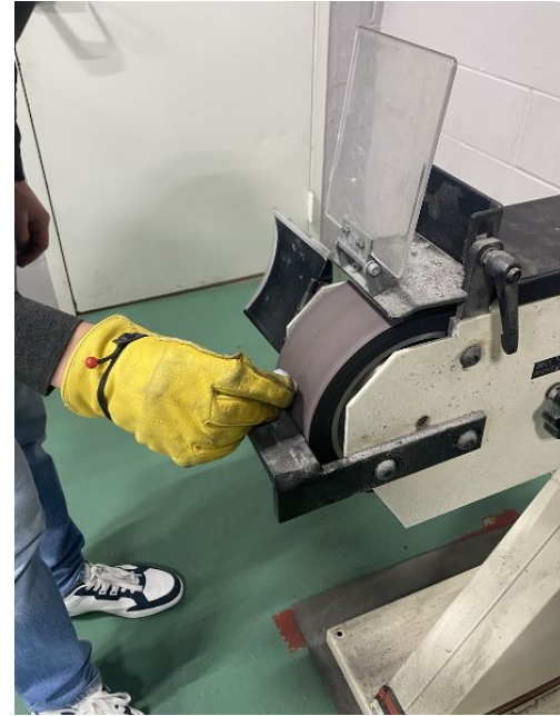
Used the sanding wheel to smooth rough edges made on the base
